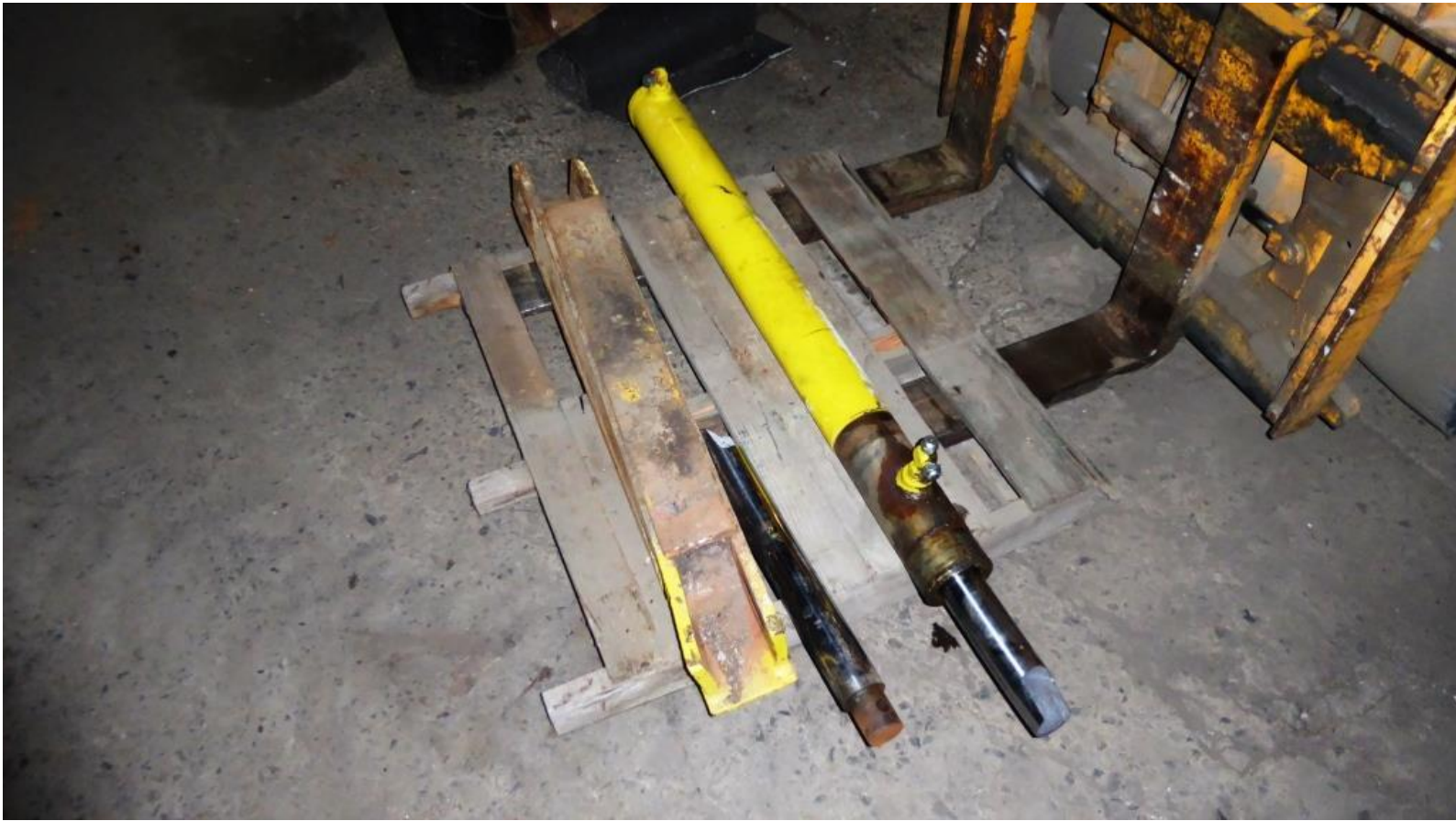
The removed broken cylinder-piston and twisted lifting ram
